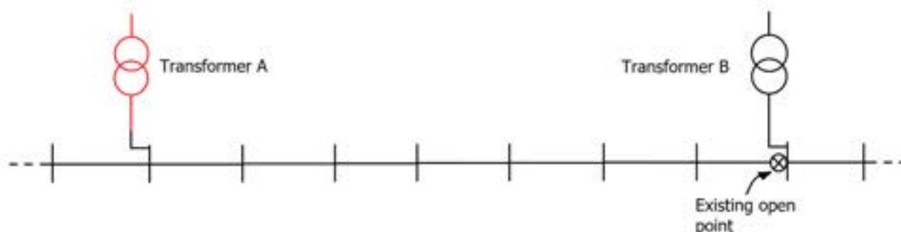
Figure 10 – Existing LV area in which transformer A is overloaded
