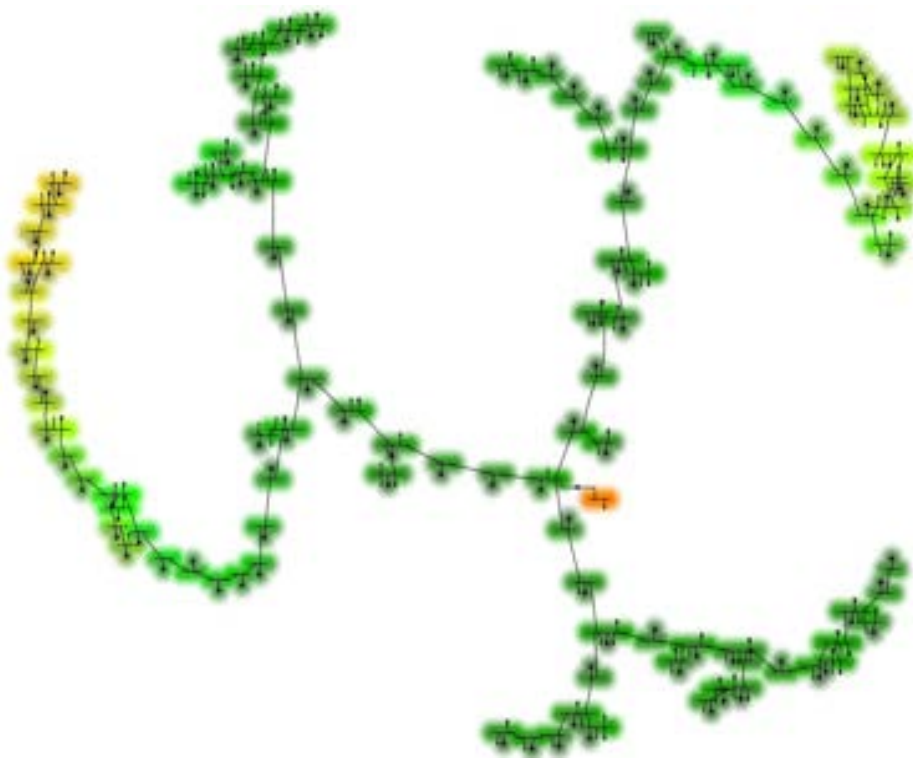
Figure 18 – Voltage magnitude heat map of one of the LV areas in the network model at noon in spring given 5 kW per household of average PV density, 50% compliance with AS4777.2 and three 50 kVA LV STATCOMs applied in this LV area (red corresponds to 250 V maximal phase to neutral voltage while green corresponds to 240 V maximal phase to neutral voltage)
