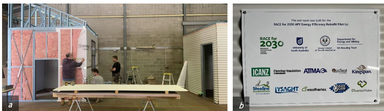
Figure 11. (a) Two 3 m x 3 m test rooms were built in Adelaide, mimicking the construction of houses in the APY Lands. (b) They were made possible through the support of industry partners and donors of materials: ICANZ, Fletcher Insulation, ATMA, OptiSeal, Kingspan, Steeline Mt Gambier, Lysaght, Weathertex, Neata Glass, and Efficiency Matrix.
