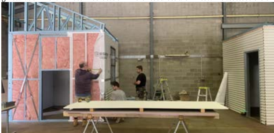
Figure 6. Two 3 m x 3 m test rooms were built in Adelaide, mimicking the construction of houses in the APY Lands. They were made possible through the support of industry partners and donors of materials: ICANZ, Fletcher Insulation, ATTMA, OptiSeal, Kingspan, Steeline Roofing Mt Gambier, Lysaght, Weathertex, Neata Glass, and Efficiency Matrix.
