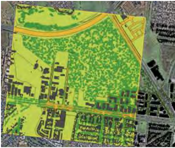
Figure 2.24. Energy Park design and thermal performance. (a) the design based on the base case scenario, (b) the air temperature during the hottest hour at the pedestrian level in 2025
