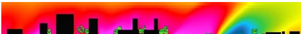
Figure 2.12. A section illustrating the air temperature at 3 pm during the hottest day in 2050. The section scale ratio in the height-to-width is 3:1
