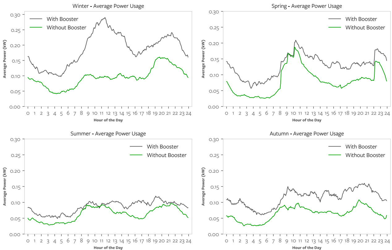
Figure 12. Average power consumption versus time of day across all monitored heat pump water heaters for each season, with and without boosters. Numbers of units with operating boost elements are 26 (winter), 22 (spring), 27 (summer) and 20 (autumn).
