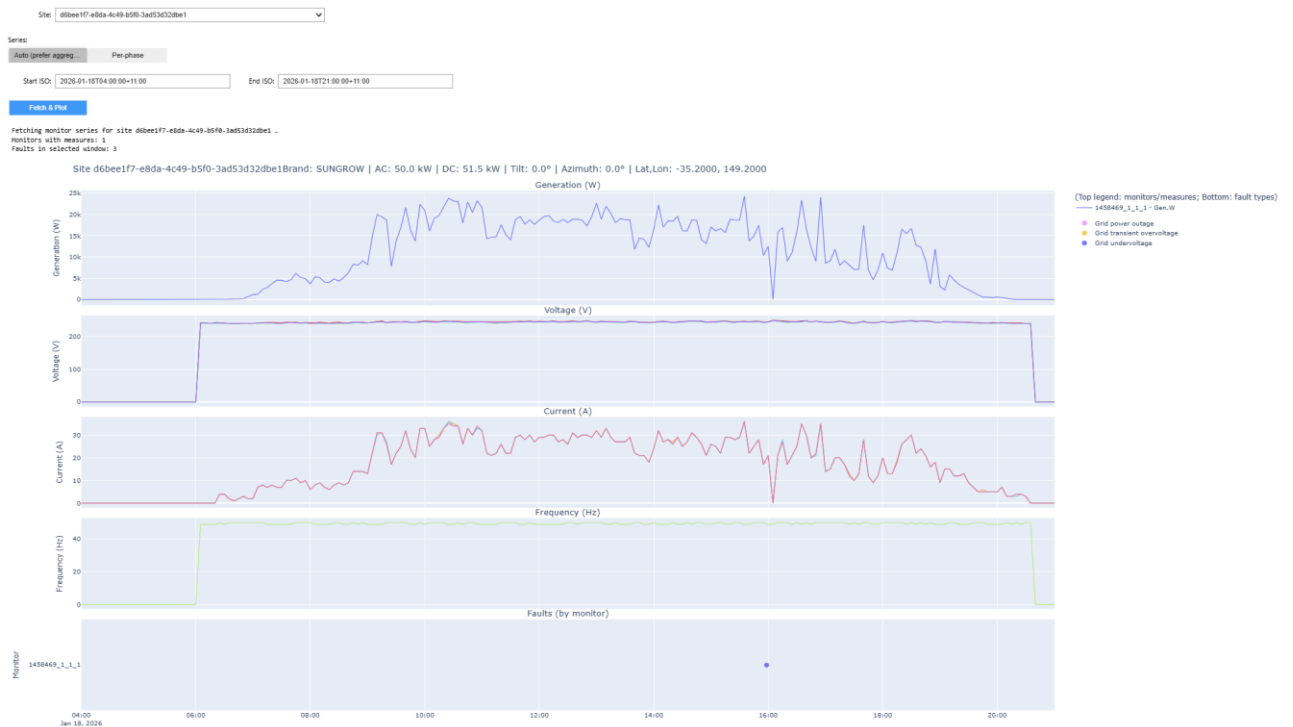
Figure A.5 for an example of a 5-minute power signal fault-inference overlapped with a fault-code retrieval.
