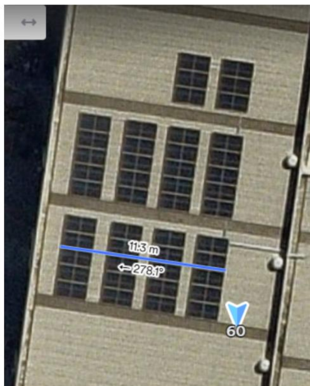
Figure A.4: Tilt and azimuth optimisation results validated against Nearmap image. Scatter plots show strong correlation between measured and predicted DC power for two MPPTs. Optimised azimuth values closely match the actual panel orientation visible in the satellite image (right).
