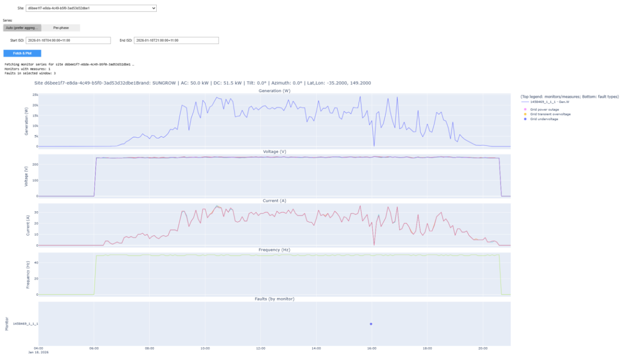
Figure A.5: Dual-method event detection using 5-minute power data and inverter fault logs. The sudden drop in AC generation coincides with a grid undervoltage fault.
