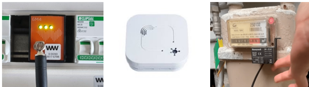
Figure 3. (1) Wattwatchers device installed in a switchboard (Source: Wattwatchers), (2) Tether EnviroQ, (3) Gas pulse monitor (Source: Tether).
