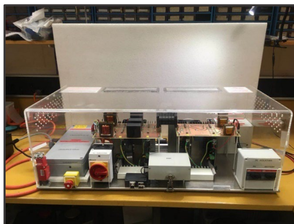
Figure 8. Prototype of the bi-directional EV charger developed at Griffith University
